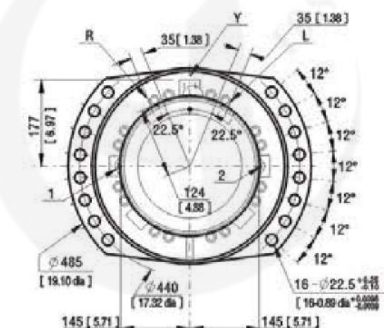
Dimensions for standard(1110) 2-displacement motor (1110) 标准双排量马达尺寸
